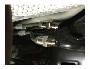
Connect the line bracket using the 2 bolts removed from the bracket (#11 on the exploded diagram above) and the supplied large diameter aluminum spacer. The spacer will go between the top bolt and the tow hook mount.
