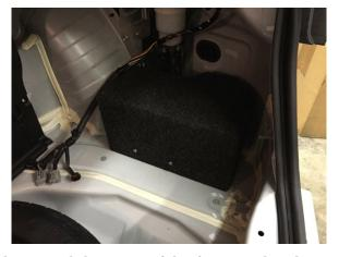
vehicle and line it up with both the trunk liner, and the seam of the frame rail and **push the bolts** as far towards the rear of the car as you can. This should slide the mounting bracket as far back as possible while keeping the pump cover in the correct location. **CAREFULLY** remove the two bolts from the cover, and gently
